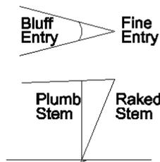
Figure 1 - Preservation of Reserve Buoyancy at the Cost of Hull Resistance
